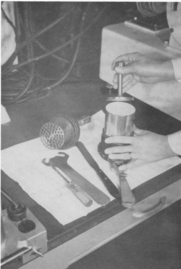
FIG. 3. An illustration of the shortening sample about to be transferred to the grease worker by means of a piston.
