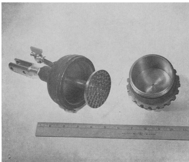
FIG. 1. The A.S.T.M. Grease Worker, modified with a vent in the bottom to allow loading of solid cores of shortening.
